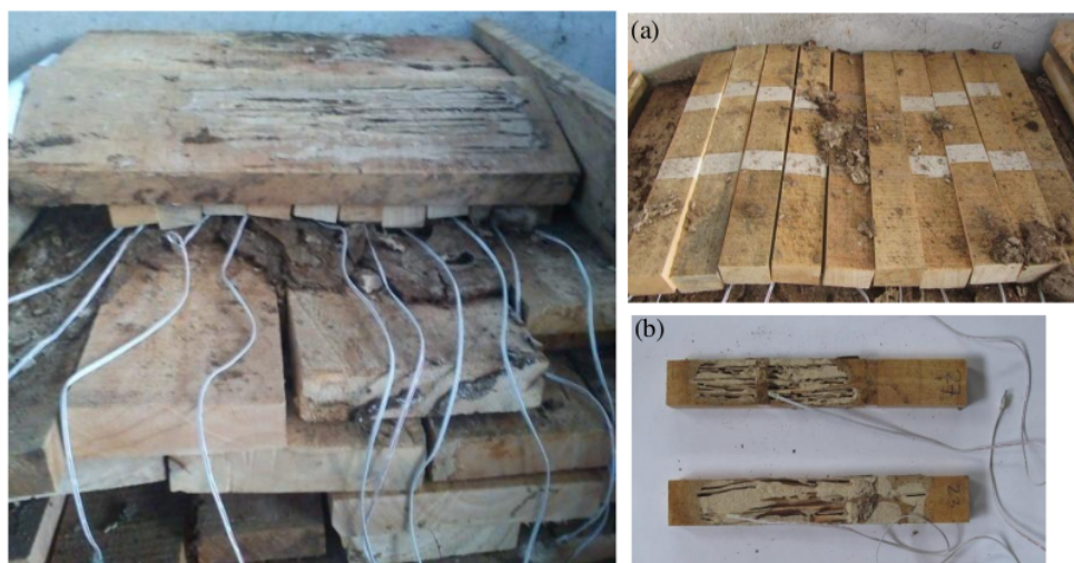
Figure 3. Wood bait installation inside Wood Drying Laboratory Forest Products Research and Development Center P3HH-Gunung Batu, Bogor, West Java, Indonesia in a horizontal manner (a) and subterranean termites Coptotermes curvignathus wood bait condition (b).
