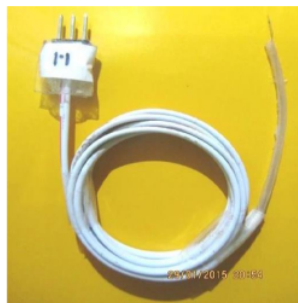
Figure 1. Thermocouple instrument used to measure the temperature in this study.
